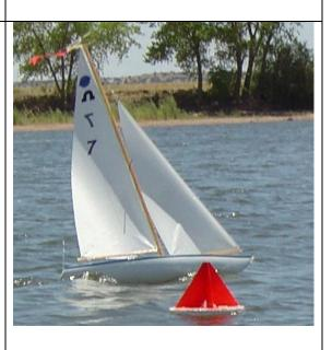
The Soling One Meter (Soling 1m) class philosophy is to provide a low-cost model suitable for introducing newcomers to the hobby while offering enough performance to keep long-time model sailors interested. The hull and deck are vacuum formed styrene plastic, the spars are wood, and the sails are flat and unpaneled.
